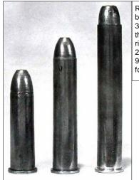
Regardless of exact caliber basic brass usually came 3% inches long such as the .50-140 cartridge at right. Then it could be cut to 2% inches to make the .50-90 at center or to 1% inches for a .50-70 such as at left.
