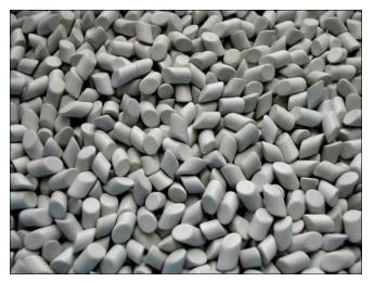
Close-up of the ceramic chips after rinsing and overnight drying  $\ldots$  these measure 4 mm x 5 mm and have their ends cut at an angle to assist with the cleaning and polishing process. This size produced no "jamming-up" inside the cases.
