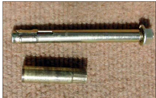
The expanding Rawlbolt seen next to the remains of the sheared-off brass case. The rifling can clearly be seen.
