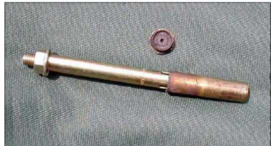
The bolt fully expanded into the case just after being tapped out of the barrel.
