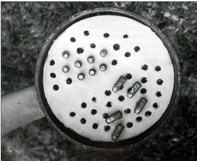
Some reloaders prefer to pan-lube their bullets wherein melted lubricant is poured around them. This method works well for bullets that come from the mould at the proper diameter.
