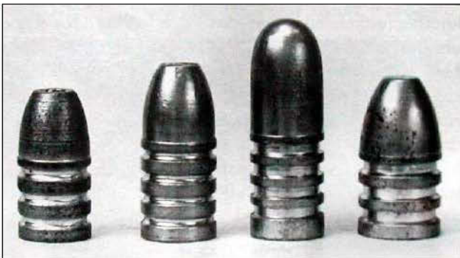
These four Lyman cast bullet designs have been around for over 100 years. From left they are: #457122 (336 grain HP), #457193 (420 grains), #457125 (520 grains), and 515141 (450 grains). All weights are for 1-20 alloy.
