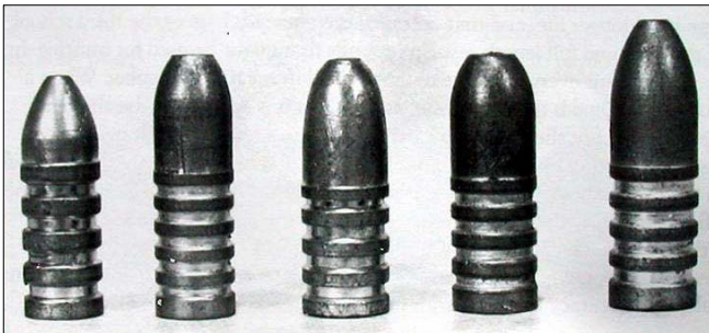
Bullets for black powder reloading should have wide and deep grooves, and their dimensions on both nose and body must fit the rifle in which they'll be fired. Over the years the author had all these custom moulds built. From left they are: Old West 366 grain .40 caliber, Hoch 410 grain .40 caliber, Tom Ballard 465 grain .44 caliber, Hoch 500 grain .45 caliber, and Hoch 550 grain .45 caliber.
