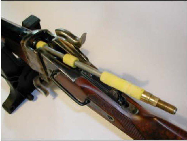
Fitting it - Nothing could be easier, just slide it in. Note the threaded end with the 2 knurled nuts to adjust head spacing.
