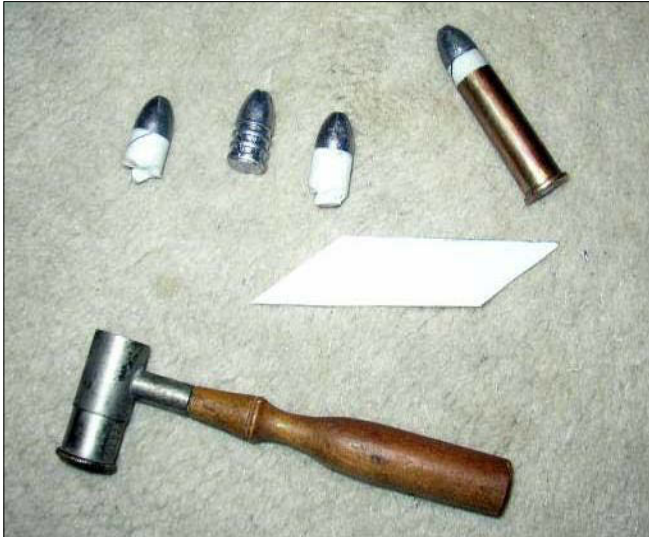
Both weights of patched bullet and grooved Government bullet from original mould, together with a loaded round.
